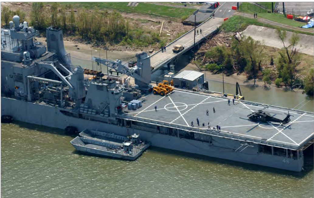
An aerial view of the dock landing ship Tortuga (LSD-46) docked outside the city of New Orleans during Katrina relief operations. Note the helicopter on one of the ship’s two landing spots and the two LCUs (landing craft utility) rafted to the port side of the ship. (NARA, 311-MAD-19211)
