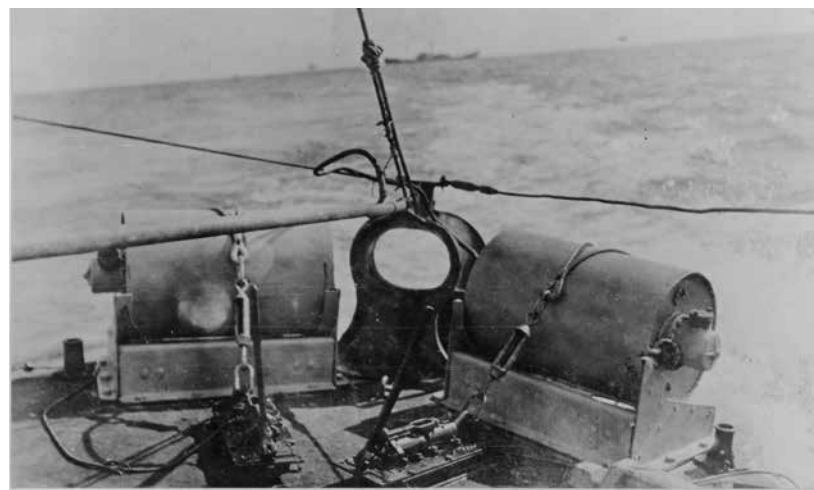
Depth charges fitted onto McCall (Destroyer No. 28) after the ship’s arrival at Queenstown, Ireland (NHHC, NH 123838)
