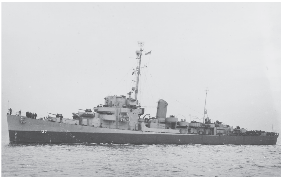
Newly commissioned Herbert C. Jones (DE-137) carried electronic jamming equipment to counter the Luftwaffe's glide bombs (National Archives and NHHC, 19-N-77794).
