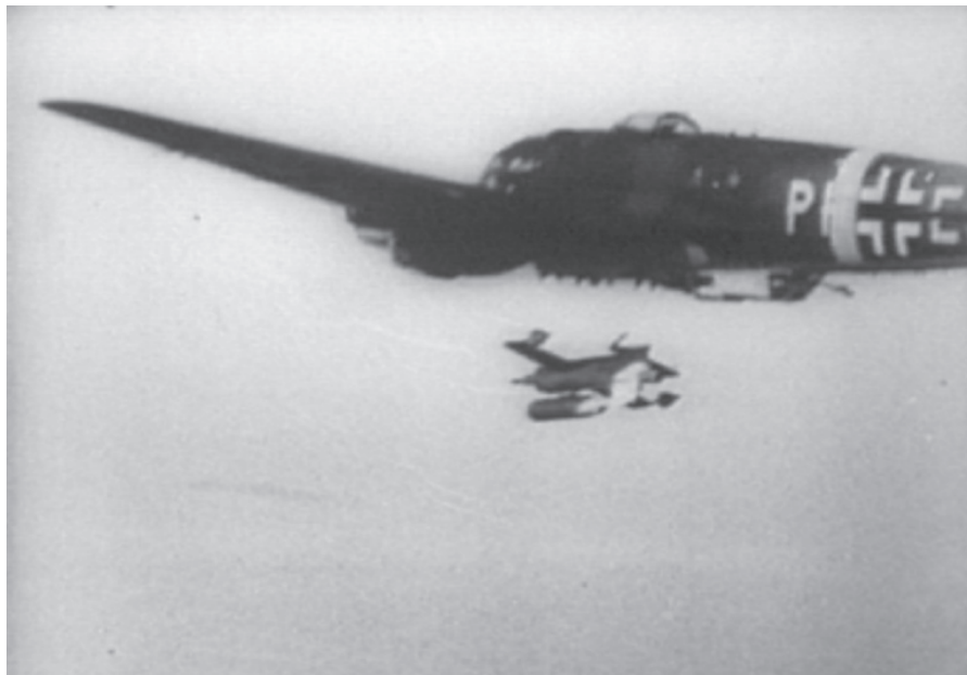
Still from a captured German film showing a Heinkel He-111 releasing a Henschel Hs-293 glide bomb (National Archives, 78193).
