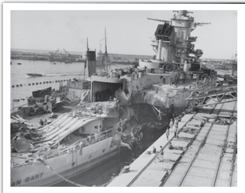
The incomplete French battleship Jean Bart at Casablanca on 16 November 1942, showing damage from 16-inch shells and 1,000-pound bombs inflicted in action with U.S. Navy forces on 8 November. National Archives 80-G-31605
