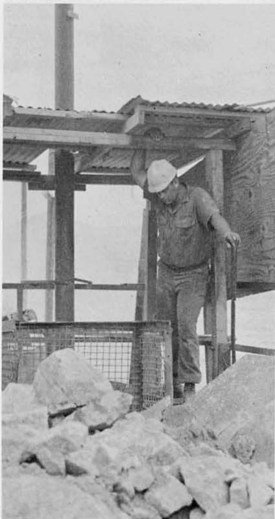
Crusher boss determines amount of rock entering crusher.
